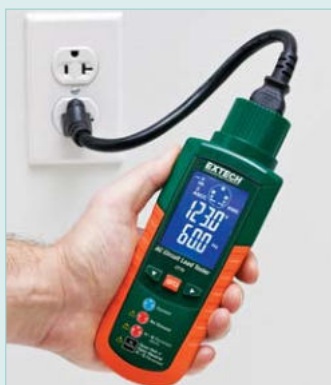
Tests 3-wire standard and GFCI receptacles
