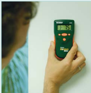
Measure moisture of wall material with non-invasive Pinless technology
