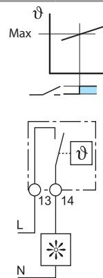
**Heating control** - Should the panel temperature fall below the (minimum) set temperature the contact will close to call for heat. The contact will open when this set temperature is exceeded.
