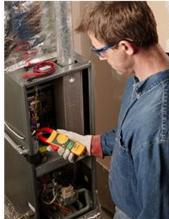
The new Fluke 902 True RMS HVAC Clamp Meter provides the accuracy, reliability and ruggedness that define Fluke test tools. It is designed for HVAC technicians for the systems they service and install daily. With True RMS technology and a CAT III 600V rating, HVAC technicians can troubleshoot and maintain HVAC equipment safely and with confidence in the results.
