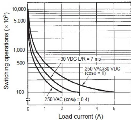
Reference: A maximum current of 0.15 A can be switched at 125 VDC ( $\cos\phi = 1$ ) and a maximum current of 0.1A can be switched at 125V DC and  $L/R = 7$ ms. In both cases, a life of 100,000 operations can be expected.
